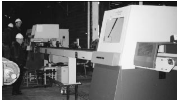
. . . with addition of new Dimter optimized chop saw line.
