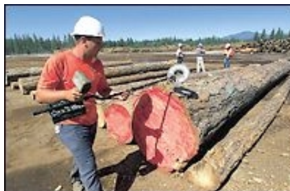
ALL WOOD ALL THE TIME: Brian Campbell checks logs with a metal detector. A nail in a log can destroy a saw blade.
